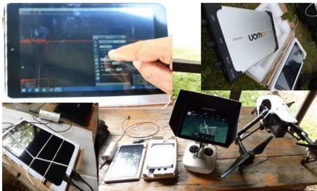
Pic 6, “Flying lab”: VF-Broadband amplifier, special /light weight/, OBD LAB, Belgrade; PC oscilloscope OWON, VDS1022; Tablet computer, I.Onik, Quad Core, Win 8.1
