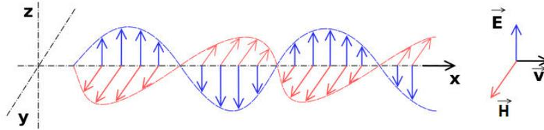
Pic.12 Conventional (“Hertzian”) electromagnetic wave
