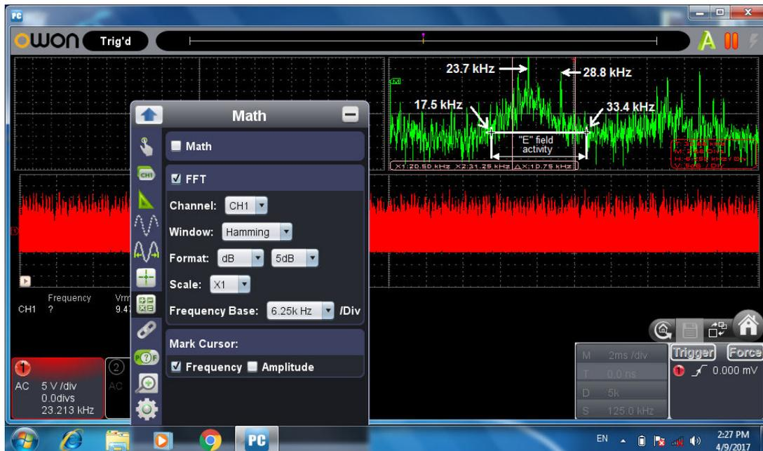
Figure 10, "E" signal in the range 0.1 - 62.5 kHz. A large electrical activity is visible in the area of 17.5 - 33.4 kHz.
