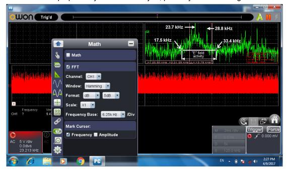
Figure 10, "E" signal in the range 0.1 - 62.5 kHz. A large electrical activity is visible in the area of 17.5 - 33.4 kHz.
