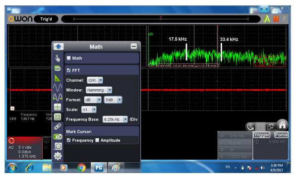
Figure 11, "H" signal in the range 0.1 - 62.5 kHz.
