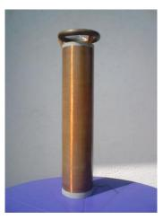
Pic 1: Classical Tesla coil Pic 1a: Classical Tesla coil in function
